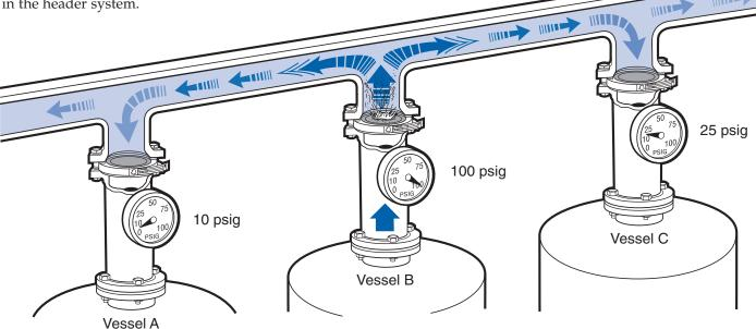
Applications of this design include: use as primary overpressure protection devices on vessels or equipment, or when mounted to the downstream side of relief valves, they provide back pressure and corrosion protection to relief valves.
