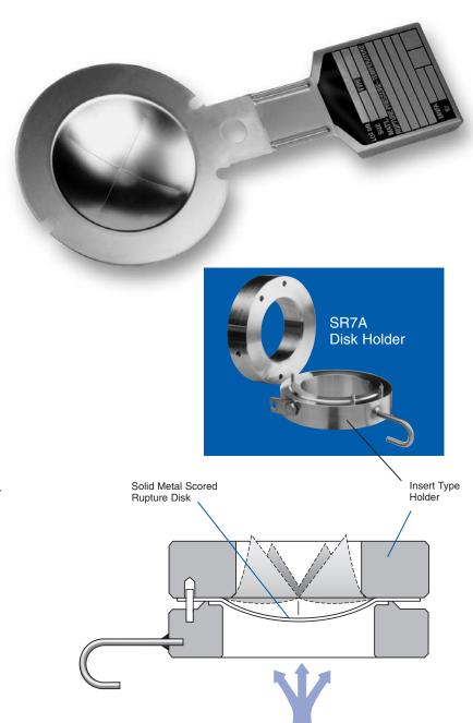
SRA Series Disks mount with the convex surface facing the process media. As pressure increases above the recommended operating ratio, the compressive stress in the disk material increases until a point of instability is reached. At that point the disk begins to buckle. It tears along the score lines as it reverses, which initiates the complete rupture of the disk
