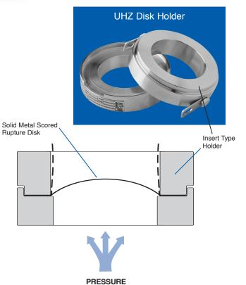
SFAZ Series Disks mount with the concave surface facing the process media. As pressure increases above the recommended operating ratio, the score lines weaken until rupture occurs. When the SFAZ Disk ruptures, the disk opens along the score lines and folds back against the holder outlet.
