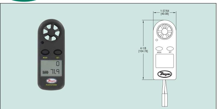
Measure wind speed and temperature with the Series MW Pocket Wind Meter. Easily view readings on the four digit 2" (51 mm) high LCD display with wind speed bar graph. Selectable air velocity ranges include m/s, ft/min, km/h, mph, and knots. Ambient temperature recorded in °F or °C. The MW also features automatic shut-off, detailed instruction manual and protective plastic water resistant housing that floats. Accessories include a lanyard.
