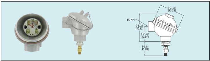
The Model A-709 Temperature Enclosure can be used to mount our Series 651 and 659 Transmitters to any of our 1/8″ diameter temperature sensors. The screw on enclosure core can be quickly removed and has a chain to prevent it from getting lost. The Model A-709 comes with the necessary adapters and fittings for attaching the temperature sensor.
