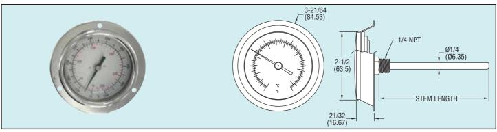
Series BTPM Panel Mount Bimetal Thermometers are designed to easily mount in most instrument panels. The front flange has three 5/32 diameter holes to quickly attach the thermometer to the panel. The Series BTPM thermometer has a dial with a scratch resistant glass lens. The Series BTPM Panel Mount thermometers are ideal for HVAC, automotive, and food industry applications, chemical operations, and more.
