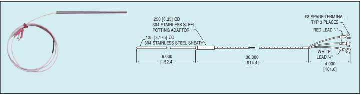
**Precision RTD** (Resistance Temperature Detector) offers excellent accuracy and stability over a wide temperature range. Industry standard 3-wire 100 ohm (DIN) probes are available in 6 " (15 cm), 12 " (30.5 cm), or 18 " (46 cm) sheath lengths with 30 " (76 cm) extension cable and spade lug terminals.
