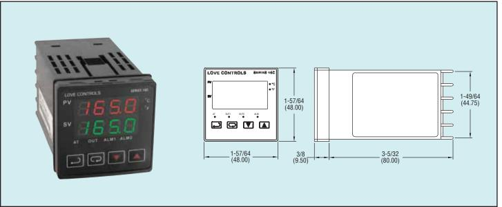
The compact Series 16C Temperature Controller offers accurate temperature measurement and control in a 1/16 DIN package. Designed for direct or reverse acting (cooling or heating) control, the Series 16C can be programmed for simple ON/OFF or more complex PID control functions. PID control is supported with manual or auto-tuning. Select relay, voltage or current output for control methods.
