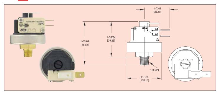
Series A9 Pressure Switches are designed for controlling pressure with higher current capacity. These switches are used widely in steam cleaners, steam irons, and other pressure control systems. It provides SPDT contact and Series A9 Pressure Switches utilize high-quality miniature snap-action switches. The switch is diaphragm operated, boasting a high temperature rating and compact size.
