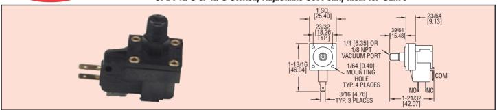
Compact, lightweight, and adjustable, the Series MVS Miniature Vacuum Switch is specially designed for OEM applications. This low cost switch has a minimum life expectancy of 10 million cycles and has an extremely fast response time. Typical applications for the MVS are HVAC, home appliance, dairy systems, medical, office equipment, and pump control.
