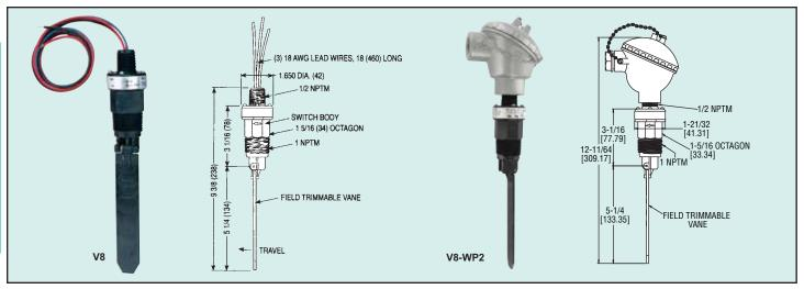
V8 Flotect® Flow Switch Protects Equipment: Operation is simple and dependable. In most applications, the switch is normally off while there is sufficient flow of liquid or air. When flow stops, the vane spring moves the vane, actuating a single pole double throw switch rated 5A @ 120/250 VAC to start or stop motor, pump, engine, etc. Operate a damper or valve; shut down a burner or actuate an alarm or signal, protecting unattended equipment from damage or loss of production.
