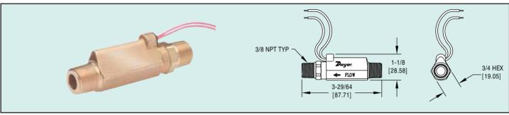
**High inline pressures** are no problem for the Series P8 brass flow switch. The switch integrates a one-piece magnetic PPS composite piston to handle pressure up to 1500 psi. The P8 switches use 100 micron filtration and are less susceptible to clogging than other high inline pressure switches. Setpoints range from 0.25 to 2.0 GPM for liquid flow. Use the Series P8 in industrial cleaning equipment or high pressure lubrication systems.
