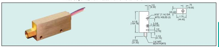
The Series P1 Brass Flow Switch utilizes a piston-type design for accurate detection of excessive or insufficient flow rates. The piston magnetically actuates a hermetically sealed SPDT reed switch. The switches have preset actuation points from 0.10 to 1.5 GPM for liquid flow. The Series P1 is ideal for protecting against loss of fluid flow in hydraulic systems or assuring proper coolant flow in semiconductor processing.
