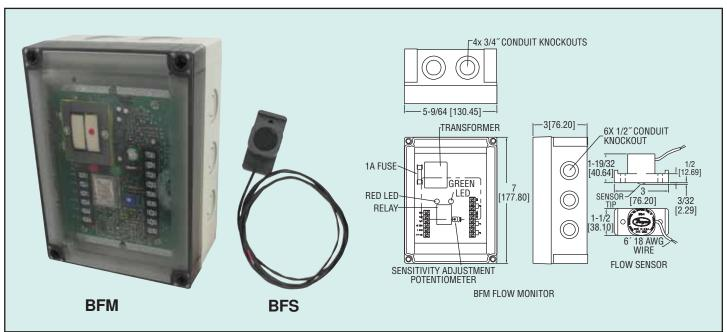
**Series BFM Bulk Flow Monitor** provides effective monitoring for most flow/no flow conditions in pipes and chutes. It's sensing techniques, which use a Piezo element, makes the BFM versatile for most flow/no flow applications.
