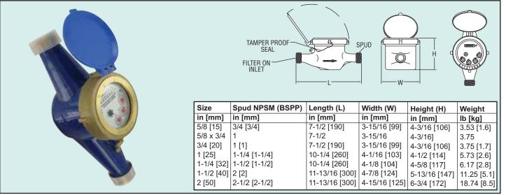
The Series WM Multi-Jet Water Meters are ideal for commercial and industrial applications. The multi-jet design allows simplicity and accuracy with wide flow ranges, even in low flow applications. The magnetically driven, hermetically sealed register will not leak or fog and is completely separated from the water. These water meters are designed for long service life and maintenance-free operation.
