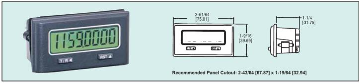
Monitor flow rate or total flow with Model TM2 Flow Totalizer. Unit features a four digit flow rate display and an eight digit totalizing display with a programmable, five position decimal point. Easily toggle between rate and total with front-panel push-button. Use scaling factor to define flow rate in engineering units such as ml/min, l/min, or gal/hr.
