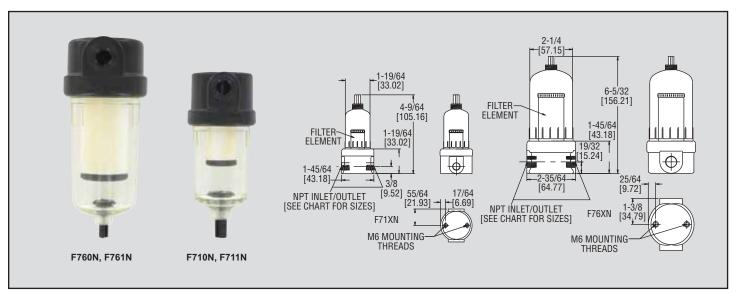
The F700 Series of filters is ideal for the filtering of liquids or gasses in low pressure systems. The nylon construction is resistant to harmful components often found in sample streams. Replaceable filter elements remove particles and droplets as small as .01 micron with 95% efficiency.
