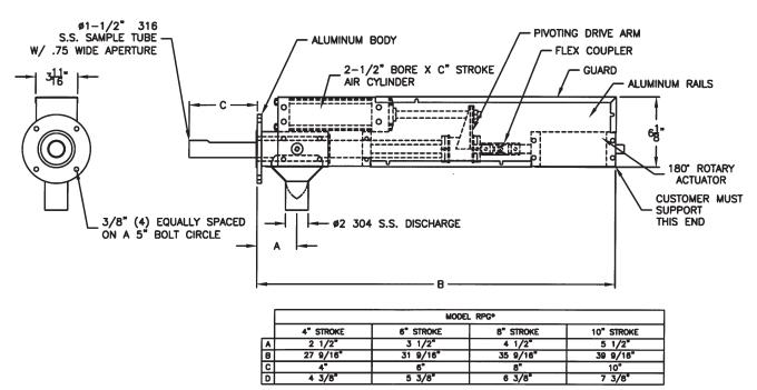
MODEL RPG MEASUREMENTS VARY, CONTACT FACTORY FOR ADDITIONAL AND/OR DIFFERENT STROKE DIMENSIONS IF REQUIRED
