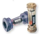
The Series IS/PX/TX Insite™ Air/Liquid In-Line Flowmeter is available in a variety of materials including PVC, aluminum, brass, or 316 stainless steel. The variety of optional materials allows the flowmeters to be used in many different applications. The Series IS/PX/TX Insite™ flowmeters are also available with an optional field adjustable reed switch for high and low alarms.
