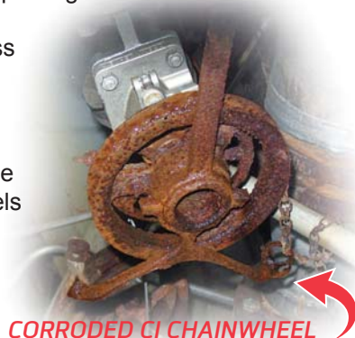
CORRODED CI CHAINWHEEL shows advantage of stainless
