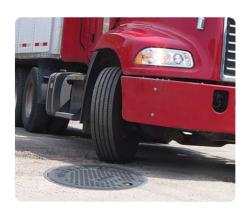
TRUMBULL POLYMER MANHOLE LIDS are today's smart choice for highway use in place of cast iron lids. They have been successfully tested to a 40,000 lb. proof load per AASHTO M-306, H-20. Test report from independent lab is available upon request.
