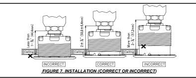
If the ceiling is to be repainted after the installation of the sprinkler, care must be exercised to ensure that the new paint does not seal off any of the air gap. Factory painted cover plates must not be repainted, they should be replaced, if necessary, by factory painted cover plates. Non-factory applied paint may adversely delay or prevent sprinkler operation in event of a fire.
