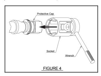
Use the "tolerance limit of back-wall level" indicator on the Protective Cap to check for proper installation depth (Ref. Figure 3) Relocate the sprinkler fitting as necessary. If desired the Protective Cap may also be used to locate the center of the clearance hole by gently pushing the back wall material against the center point of the Cap.
