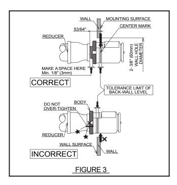
With pipe thread sealant applied to the pipe threads, hand tightens the Sprinkler into the sprinkler fitting.
