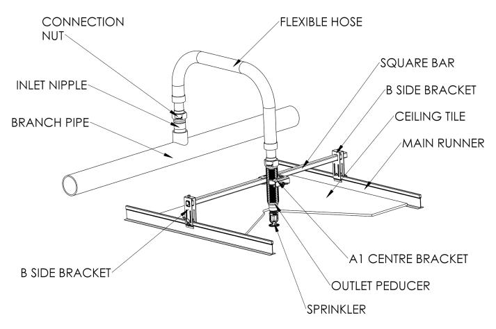
1. Install the Inlet Nipple in the branch pipe outlet using the normal sealing and tightening methods for connecting pipe threads. Tighten firmly with a pipe wrench for leak proof connection.
