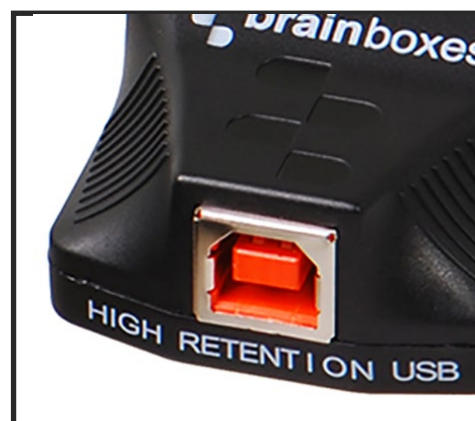
High retention USB connection requires a minimum withdrawal requirement of 15N (thats a force of 1.5Kg or 3.4lbs)
