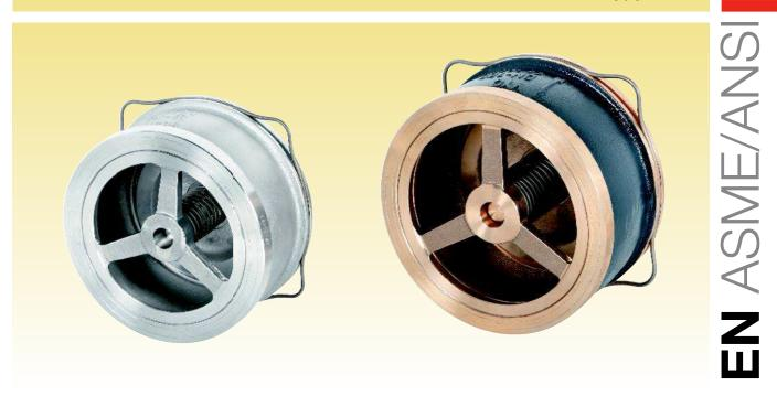
Disc check valve with centering ring for placing between flanges in accordance with DIN, UNE, ANSI, BS, etc. norms. DN-125 to 200 (DN-15 to 100 see catalogue for Model 170).
