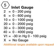
**Port Style** = 1/4" NPT Female All Gauge Ports are 1/4" NPT Female **Optional Features** This section can have multiple options
