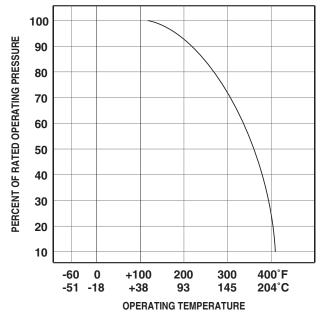
For operation at temperatures above ambient conditions, please refer to the chart above for reduced pressure
