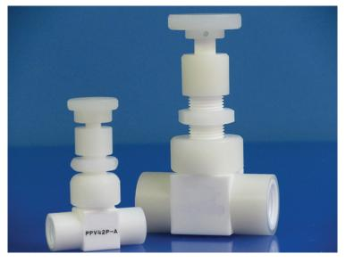
NACOM'S P.P.V (PRECISION PLUG VALVE) Series of plug valves are machined from virgin PTFE with a single rising stem and tapered plug. The basic construction is a single through orifice with a tapered body that matches the tapered plug for positive shut-off. Various orifice and port sizes are available as standard items. Additional sizes and configurations are available upon request.
