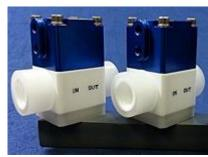
**IPS PTFE HP Diaphragm Valve (HPV)** is designed for use in high purity water and aggressive chemical applications. Designed with a 100% virgin PTFE wetted flow path, the unit is ideal for DI Water Systems and corrosive media found in solar, semiconductor, pharmaceutical and chemical process applications.
