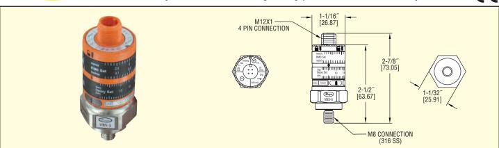
The Series VBS Vibration Switch is small, compact, and uses two easy set up dials that adjust the maximum RMS velocity set point and false trip time delay. The Series VBS is intended to continuously monitor the changes in a machine's vibration level. The VBS takes real-time RMS vibration input and provides an analog output of velocity as well as a switching output when an alarm value is exceeded.
