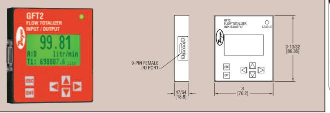
The Series GFT2 Flow Totalizer is a microcontroller driven device designed to linearize the flow meter and controller flow curve plus display the instantaneous flow rate, total, and accumulated total. The totalizer is intended to be used with analog flow meters and controllers with analog 0 to 5 VDC, 0 to 10 VDC, or 4 to 20 mA interface. RS-232 or RS-485 digital interface is available.
