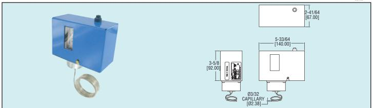
The Series DFS Low Limit Freeze Protection Switch protects cooling coils in air handler systems by preventing frost build up on the coils. By sensing the lowest temperature along any 1' section of capillary, the DPDT manual or automatic reset relays signal the building management system, as well as cut off the fan. Set points can be adjusted as low as 34°F (1° C) utilizing the visual set point indicator and set point screw. The Series DFS includes mounting clips for easy installation.
