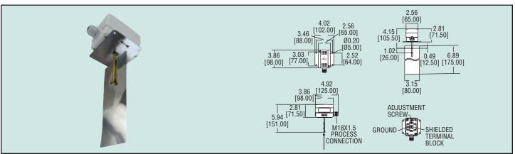
The Model AAFS-1 Adjustable Air Flow Switch is capable of detecting a wide range of air velocities with minimal user calibration. The adjustable screw changes the set point at which the SPDT snap switch engages. Quality features include a stainless steel vane, galvanized steel base, and ABS enclosure. The unit is field adjustable from 200 to 1800 FPM (1 to  $9.2~\mathrm{m/sec}$ ).
