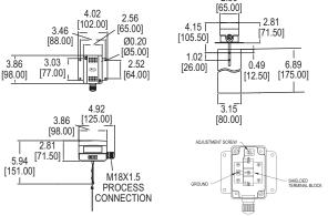
The Model AAFS Adjustable Air Flow Paddle Switch is capable of detecting a wide range of air velocities with minimal user calibration. Quality features include a stainless steel vane, galvanized steel base, and ABS enclosure.
