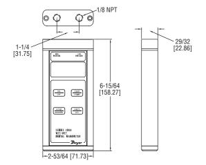
The **SERIES 490A** Digital Manometers are versatile, hand-held, battery operated manometers available in several basic ranges for positive or positive differential pressure measurement and can tolerate most liquid media compatible with 316LSS. A new feature added to the Series 490A is a field adjustable damping, which allows the user to choose the level of display averaging rate corresponding to the fluctuation level common in many applications.
