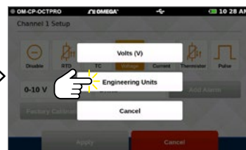
Select Engineering Units
