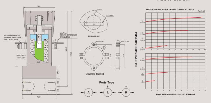
088 Series is a 1/4" and 1/2" NPT type back-pressure regulator suitable for water, chemical, liquid, gas, etc. Having Cv=0.05 or 0.6 and made of stainless steel 316L, 088 Series is specially suitable for high pressure from 5bar (72psig) up to max 700 bar (10,000psig).
