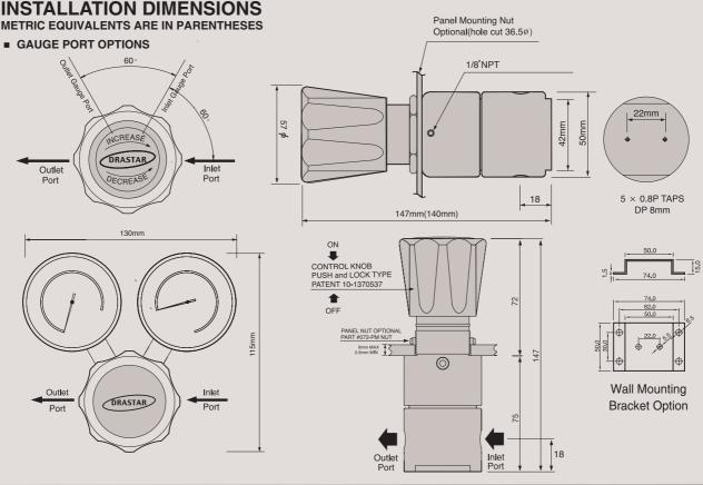
082 Series is a 1/4" NPT type single-stage high pressure reducing regulator designed to use for gas cylinder and all high pressure gases more easily and safely with "Piston-Diaphragm" which Drastar specially developed.
