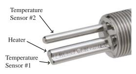
Temperature Differential = Temperature Sensor #1 Minus Temperature Sensor #2
