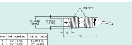
The Series TDS Thermal Dispersion Flow Switch offers solid state flow detection of non-coating liquids for pump and process protection. SPDT output allows for interfacing with remote PLC or relay control device. The adjustable switch point is factory calibrated at 0.2 fps with LED indication of flow and calibration status. Units feature selectable NO or NC operation and are not damaged by overranging flow velocities.
