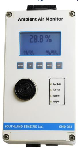
The OMD-351-O2 Ambient Air Monitor is designed to measure and assure the appropriate level of oxygen in an enclosed or confined area. Personal safety is a primary issue in nearly every industry and is magnified within confined spaces where oxygen depletion or asphyxiation due to a leak in an inert gas container can quickly and unexpectedly take place.
