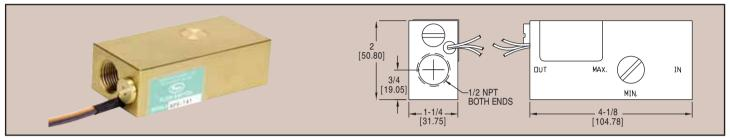
The Series AFS Adjustable Flow Switch is externally adjustable and is ideal for protecting machine tools from coolant flow failure, protecting bearings from loss of lubricant or assuring proper air flow. The Series AFS offers an infinite number of flow settings from 0.5 to 20 GPM at pressures up to 1000 psig, with low pressure drop and precise repeatability. The AFS is housed in either brass or stainless steel and can be used with water, compatible liquids, oils, and gases.
