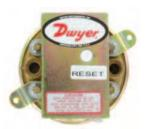
Manual reset Model 1900 MR includes special snap switch which latches on pressure increase above the setpoint. Switch must be manually reset after pressure drops below the setpoint. To order, change base model to 1900 and add MR suffix after range number. Example: 1900-10-MR. Available on -1, -5,-10 or -20 ranges only. Option is not UL, CSA or FM listed
